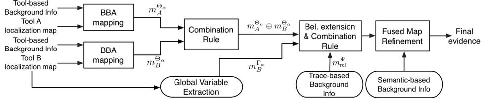
**Fig. 1.** Block scheme of the proposed framework for forgery localization, where two tools A and B searching for a forensic trace  $\alpha$  are considered. For the sake of clarity, global variables for Tool A are omitted in the drawing.
